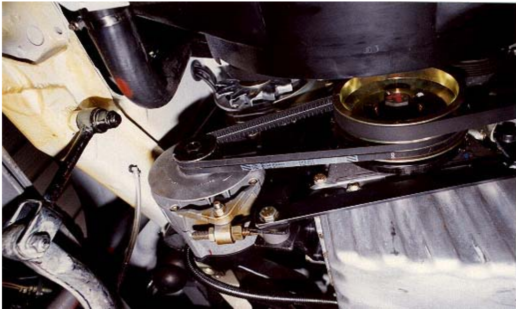
Generator Installation with 2x9,5mm B-belts
