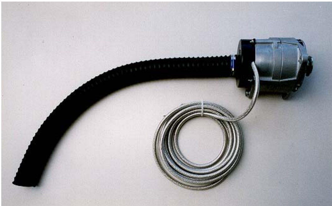
Generator with DIA 55mm air intake hose (recommended max. length 60cm) Cut any place at the rear cover for gen.cable exit
